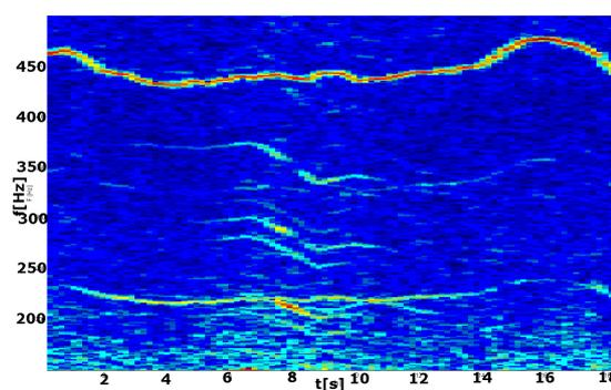
**Figure 8: Time-frequency signals of an AVS on a flying UAV during Cessna pass-by. Colour represents signal strength.**
