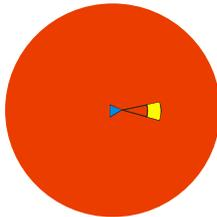
**Figure 3: Field of regard comparison acoustic (ROM 80km<sup>2</sup>, in orange) versus camera (ROM 0.3km<sup>2</sup>, in yellow).**
