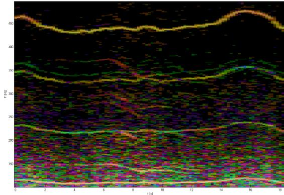
**Figure 9: Time-frequency signals of an AVS on a flying UAV during a passing Cessna. Colour indicates a DOA.**
