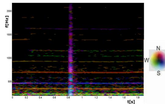
**Figure 7: DOA signals from the AVS on the UAV of 81mm HE mortar launch (approx. 500m distance).**
