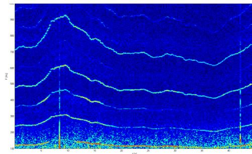
**Figure 6: Signals from the AVS on the UAV of 81mm HE mortar launch (approx. 500m distance) and impact (approx. 3km distance).**
