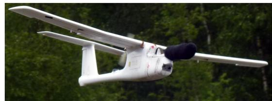
**Figure 4: A foam Skywalker with an AVS mounted on the nose, just before landing.**
