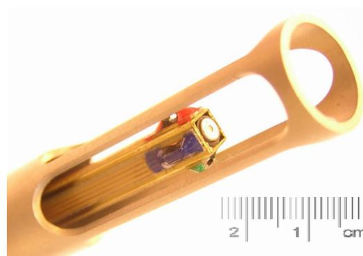
Figure 2: An acoustic vector sensor consisting of a sound pressure microphone and three orthogonally placed Microflown sensors.
