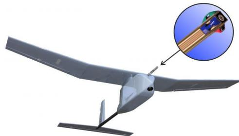
**Figure 10: The UAV DOA demonstrator. An AVS is placed on the nose and localisation results are displayed in the view of a wide angle camera.**
