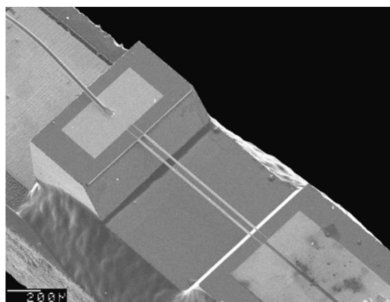
Figure 1: the Microflown sensor.
