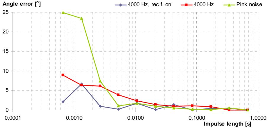
Fig. 12. Example results obtained for different kind of impulsive sounds. Noise and tonal burst with different length were used
