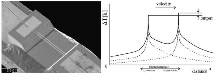
Fig. 1. (Left) A microscope picture of a standard MicroflowN. (Right) Dotted line: temperature distribution due to convection for two heaters. Both heaters have the same temperature. Solid line: sum of two single temperature functions: a temperature difference occurs [5]
