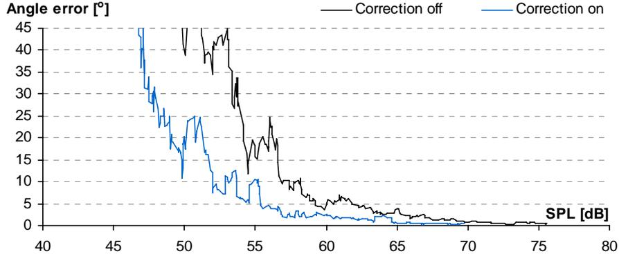
Fig 10. Example results for one third octavo band noise. Centre freq. equal to 1000 Hz
